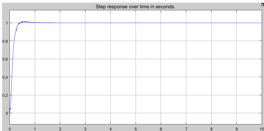
Figure 20: Step response, 0-1°, for the controller with parameters operating above 11 km/h. This was done using MATLAB.
