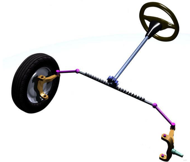
Figure 3: Illustration of a rack and pinion setup [22].
